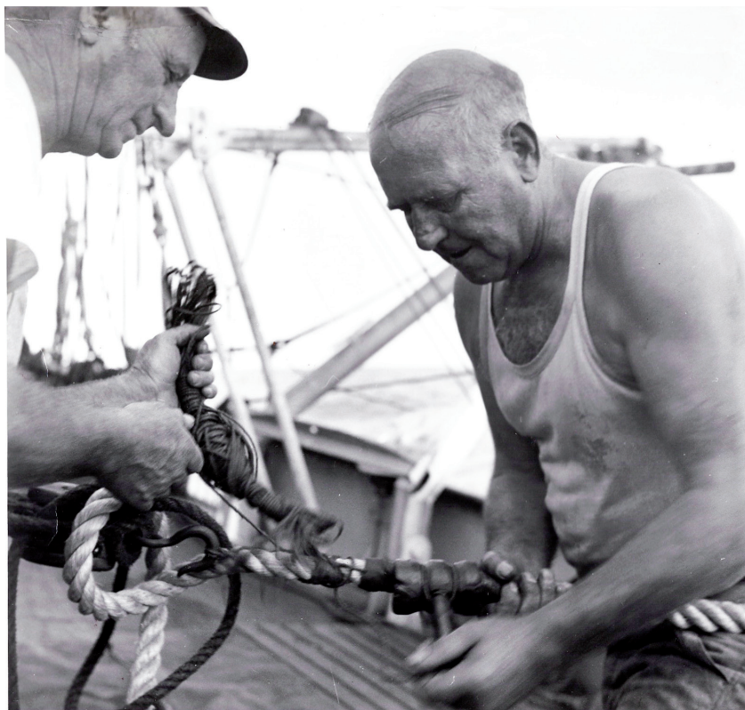
Bosun Mattie Richard and Mate Arvid Karlson putting in an eye splice aboard Atlantis . The mantra for an eye splice was Worm & Parcel with the Lay, Turn and Serve the other way. The block and tackle visible below Richard's hand holds the work taut. Arvid Karlson was a good friend and mentor aboard Atlantis . Photo by Jan Hahn.
