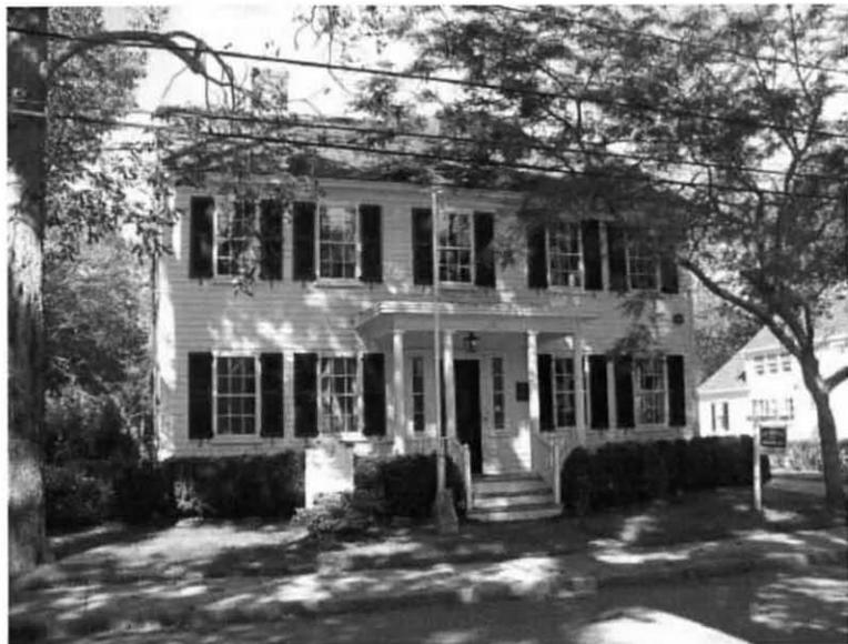
The front outside shutters were milled in David Newton's shop to match the original ones which are used in the rear of the house. All of the shutters were closed during Hurricane Irene; the wind driven rains never touched the windows. All of the windows are original to the house. Storm windows have been made to protect them and to majorly muffle all outside noises.
