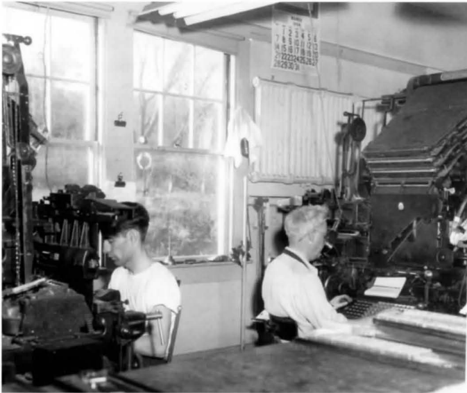
By the late 1960s The Enterprise had three typesetting machines. One was equipped with TTS or teletypesetter.
